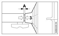
When correctly inserted, the shield (3) must be flush with the coupling sleeve (gap A must be no more than 5 mm).
