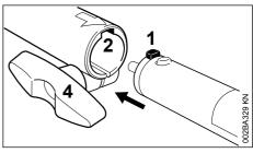
Push the pin (1) on the shaft into the slot (2) in the coupling sleeve as far as it will go.
