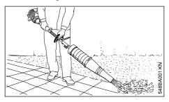
Always hold the unit firmly with both hands on the handles. Right hand on control handle, left hand on loop handle on the shaft, even if you are left-handed. Wrap your thumbs around the handles.
